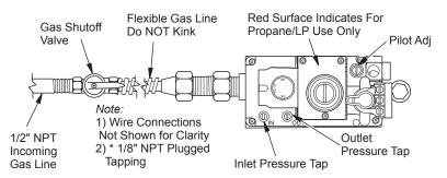
Figure 21 - Connecting Flexible Gas Line to Millivolt Valve
